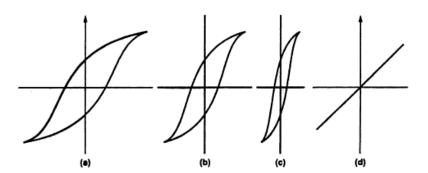
The Fig. (a) shows loop of hard steel, which is magnetic material.
