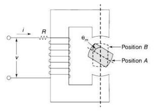
A coil is wound round a magnetic core and is connected to a voltage source. The rotor will experience a torque where the magnetic field is strong. So, the rotor will try to take a position where the reluctance of the magnetic path is the minimum. This reluctance is dependent on the rotor angle. This torque is called **reluctance torque** or saliency torque due to saliency of the rotor.
