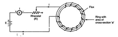
The ring specimen as a mean length of T metres with a cross-sectional area of 'a' square metres. Coil is wound for 'N' turns carrying a current T which can be varied by changing the variable resistance 'R' connected in series. Ammeter is connected to measure the current. For measurement of flux produced, fluxmeter can be used which is not shown in the figure above.
